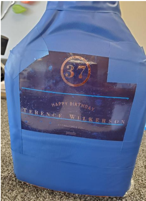
Vinyl Blasting Tape Applied
